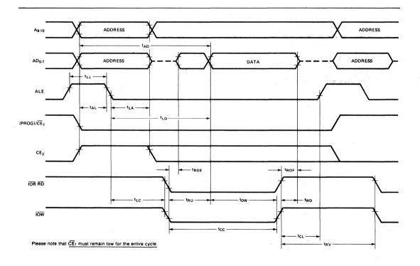
Figure 3. PROM Read, I/O Read and Write Timing
